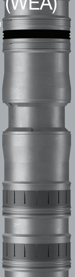
The Welltec® Expandable Anchor (WEA) for Casedhole Plug provides a temporary or permanent abandonment solution with a qualified gas-tight seal. Surface-controlled hydraulic expansion ensures bidirectional anchoring and sealing. The solution is qualified in accordance with the highest-level API and ISO standards.
